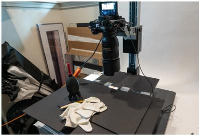
to do the same thing with my 105mm Macro lens if I thought a little outside of the box. I blew the dust off my copy stand, dug my portable light table out of the back of my closet and with a little bit of adjustment rigged up a 35mm slide copying process
